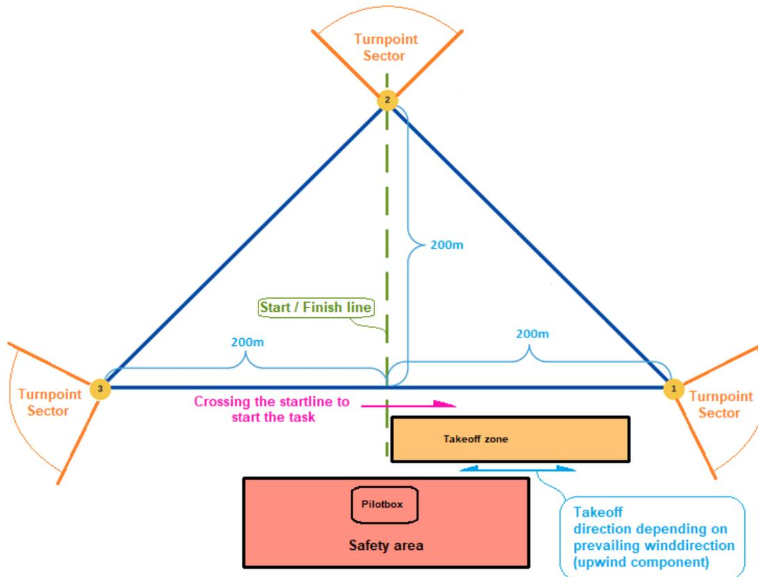
The position and the size of the Take-off Zone as well as the Security Zone may vary because of geographical circumstances of the flying field. The Take-off Zone conforms to the minimum width of 20 meters and a length of at least 50 meters. The Pilots Area's position inside of the Security Zone can be chosen freely by the contest director. The sketch above is not true to scale. The view of the area in which the triangle is placed should be unrestricted
